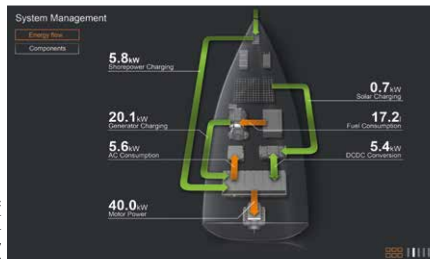
Energy flow: Understand your system's power balance and energy flow at a glance
